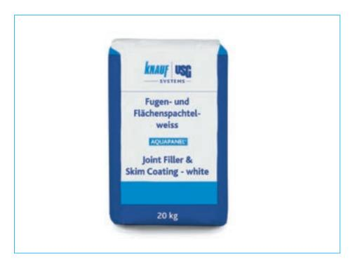
AQUAPANEL® Joint Filler & Skim Coating – white is a cement-bound filling material for full-surface skim coating to a thickness of 5 mm on AQUAPANEL® Cement Board Indoor (wall and ceiling) and AQUAPANEL® Cement Board Outdoor (ceiling), for example before the application of a decorative plaster or paint finish. For interior and exterior use.
